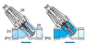
The Upstream Pressure **[P1]** applies balanced opening and closing hydraulic forces under the Diaphragm **[1]** and above the Plug **[2]**. The Downstream Pressure **[P2]** applies hydraulic closing force under the plug, which seeks to reach equilibrium with the Set Spring **[3]** force. Should **[P2]** rise above setting, the hydraulic closing forces rise above the mechanical force of the spring, pushing the plug to modulate closed, and reducing **[P2]** back to setting.
